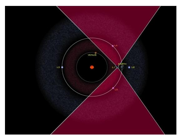
A depiction of the field(s)-of-regard of the space-based NEO survey telescope, NEOCam, located at SEL1. Optimized in the infrared, this telescope looks forobjects in the leading and trailing portions of the Earth's orbit to find and catalog PHOs.
